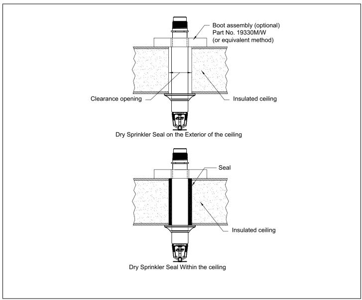
Figure 6: Dry Sprinkler Seal (Adjustable Standard Dry Pendent Sprinkler is Shown)
