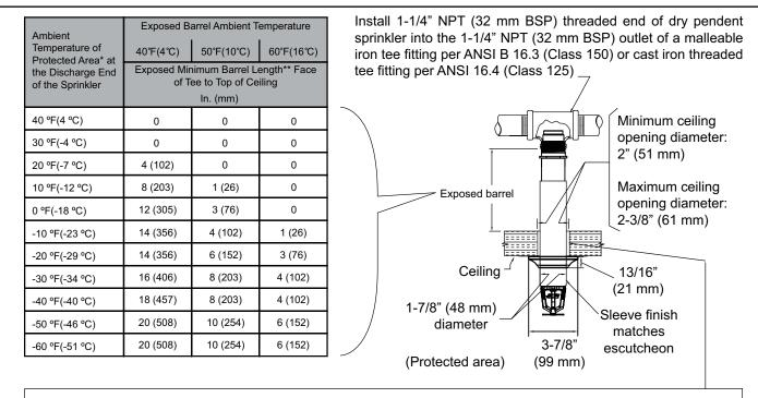
Seal the clearance space around the sprinkler to avoid leakage of air into the protected area and consequent formation of condensate around the frame, which could inhibit operation or cause premature operation. Refer to Figure 6 below.
