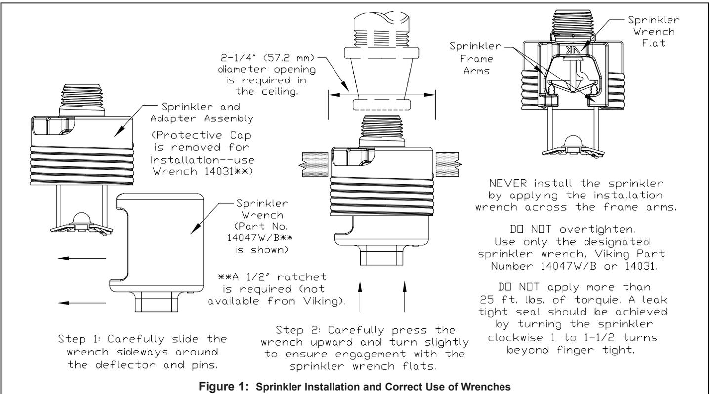
**Figure 1: Sprinkler Installation and Correct Use of Wrenches**
